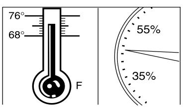
**Conditioning paper** Because temperature and humidity affect paper performance in the printer, you need to condition paper before using it. To do this, store paper for a specified length of time in the same type of environment as your printer.
